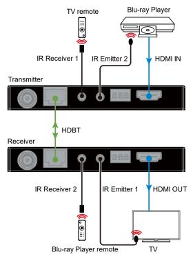
Note: Connect the broadband IR receiver to IR IN and the IR emitter to IR OUT.
